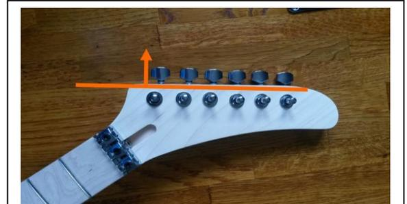
Figure 2.7 Tuner Alignment
