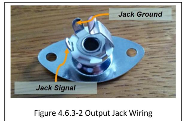
Figure 4.6.3-2 Output Jack Wiring
