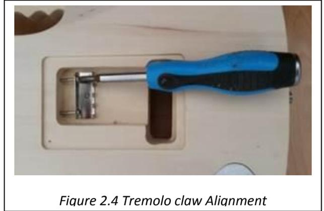
Figure 2.4 Tremolo claw Alignment
