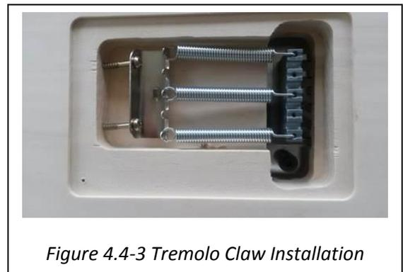
Figure 4.4-3 Tremolo Claw Installation
