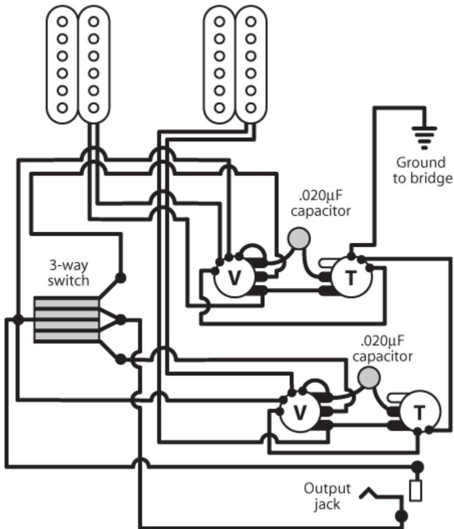
Each pickup has a wire and a ground. The bridge pickup has a white wire and the neck pickup has a yellow wire.
