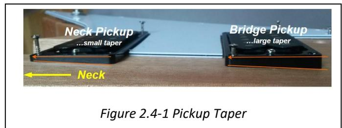
Figure 2.4-1 Pickup Taper
