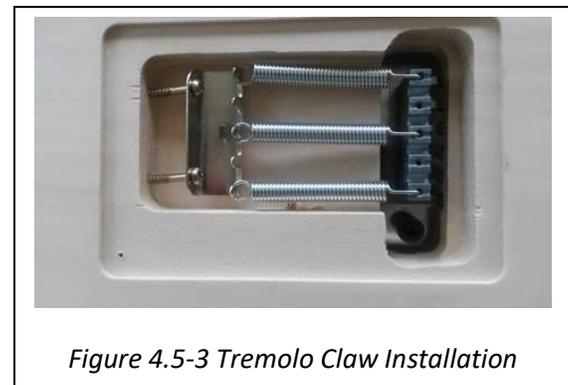
Figure 4.5-3 Tremolo Claw Installation
