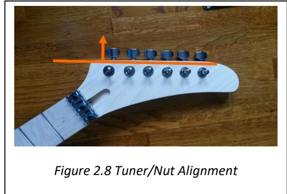
Figure 2.8 Tuner/Nut Alignment
