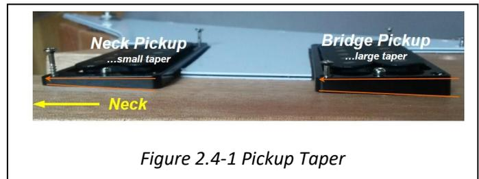
Figure 2.4-1 Pickup Taper
