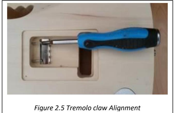
Figure 2.5 Tremolo claw Alignment
