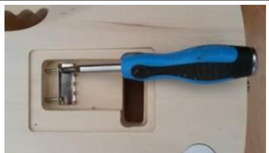
Figure 4.5-1 Tremolo Claw Installation
