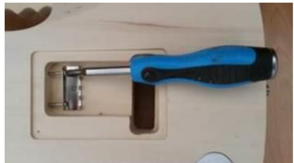
Figure 4.4.3-1 Tremolo Claw Installation
