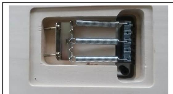
Figure 4.4.3-3 Tremolo Claw Installation
