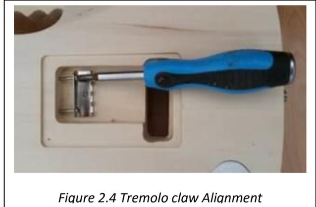
Figure 2.4 Tremolo claw Alignment
