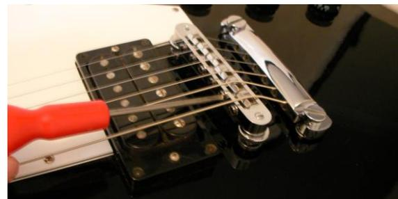
Fig 5.5 Intonation Adjustment
