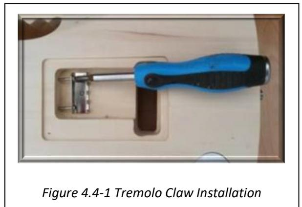
*Figure 4.4-1 Tremolo Claw Installation*
