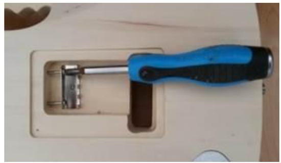
Figure 4.4-1 Tremolo Claw Installation
