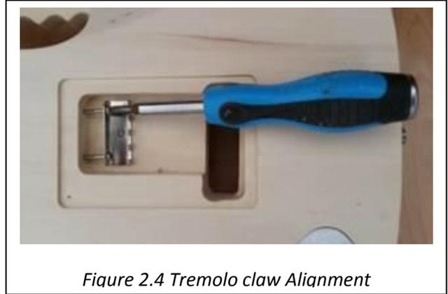
Figure 2.4 Tremolo claw Alignment
