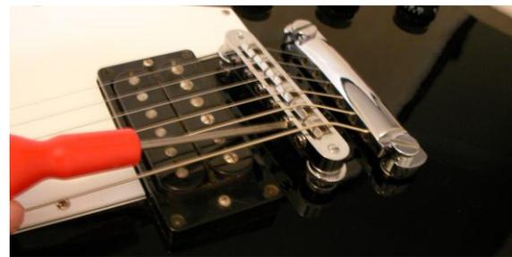
Fig 5.5 Intonation Adjustment
