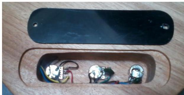
Figure 4.2.1-2 Completed Electronics Installation
