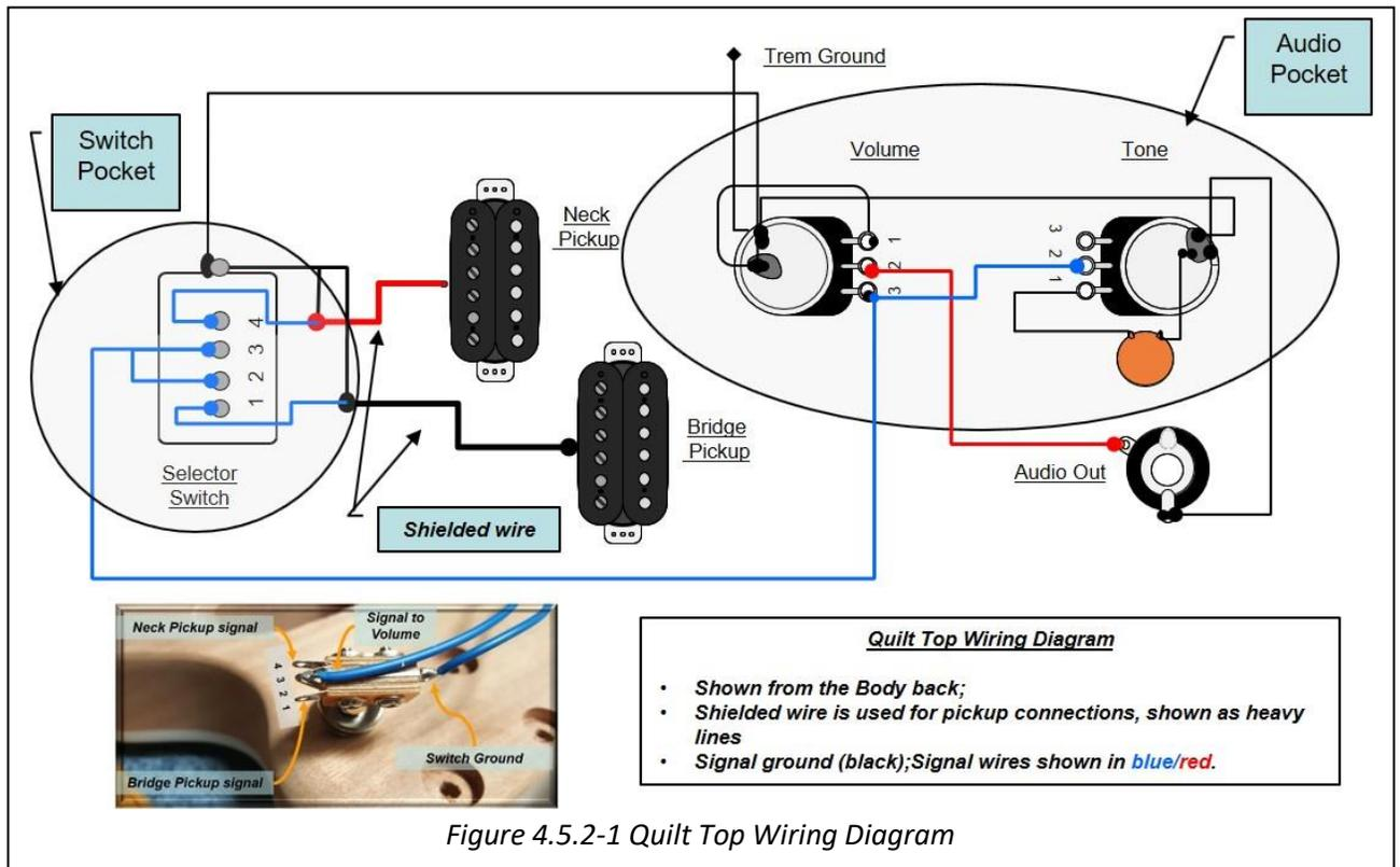
Figure 4.5.2-1 Quilt Top Wiring Diagram
