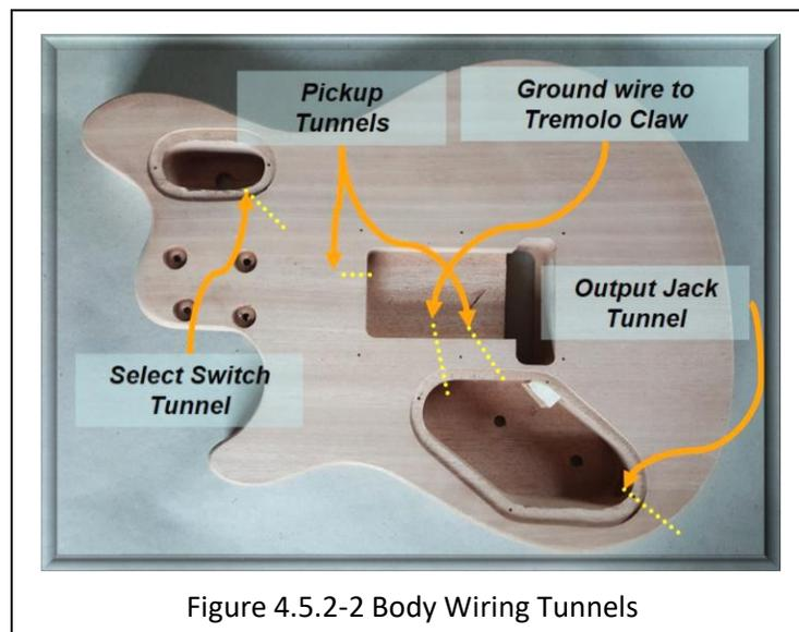
Figure 4.5.2-2 Body Wiring Tunnels
